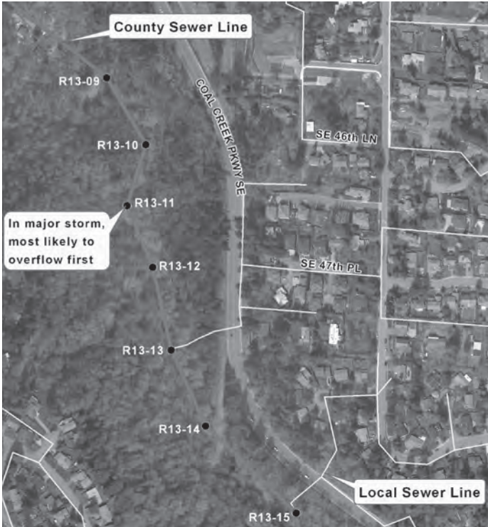
Figure 2. First manholes to check when suspecting an overflow
